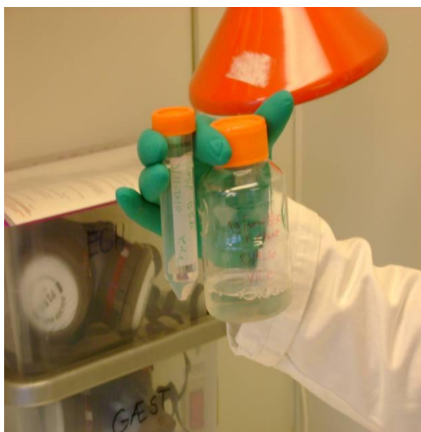
Figure 3.3 Flask with raw 1% w/v BSA solution and a 1% w/v sterile-filtered BSA-solution in a centrifuge vial. After sterile filtration the 1% w/v BSA stock solution can be kept in a refrigerator for at least 2 weeks.
