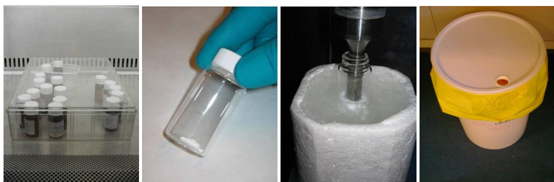
Figure 2.1 Examples of suggested good practice for storage and handling of NM. A) Storage of vials in an easy accessible transparent box. B) Handling of powder in small amount. C) Sonication of dispersions in a fume-hood. D) Discard of nanomaterial waste in a designate waste-contained for chemical waste.
