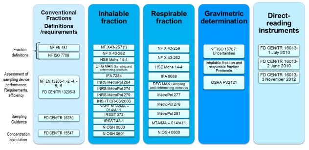
(\*) The NF X 43-257 standard does not describe the sampling of the inhalable fraction, but rather the sampling of aerosols using a cassette (4mm orifice). However, the method described in this standard is used in many countries to determine the inhalable fraction of aerosols.
